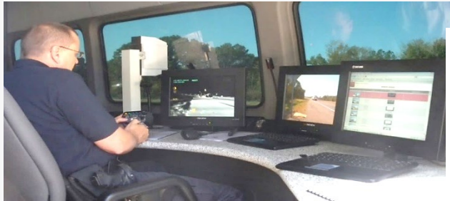
Expanded ITD capabilities may include mobile vans with camera, weight, and sensor technologies deployed to increase the effectiveness of roadside enforcement.
